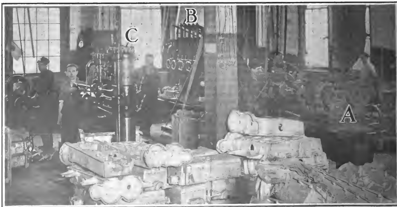
Fig. 1—General view of machine shop in National Motor Vehicle Company, showing cylinder boring machines working on gangs of engine cylinders. Crankcases are shown in the foreground
